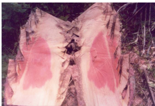
Figure 6. Dye distribution profile in the stem.
