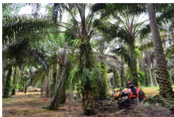
Figure 7. The tractor mounted trunk injector at work.
