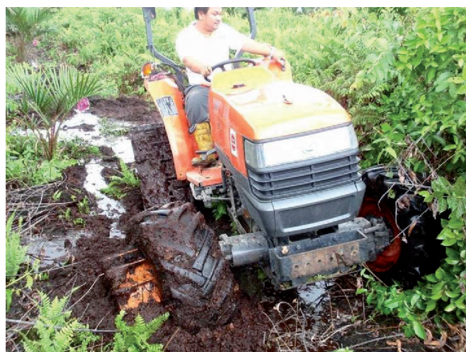
Figure 4. Crawler tractor with cage wheels and ground skid operating in peat soil.
