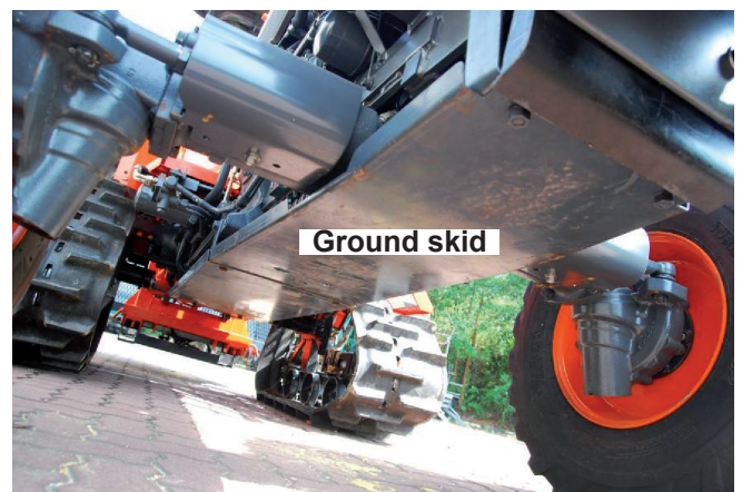
Figure 2. Ground skid to protect against obstructions for the smooth movement of the tractor.
