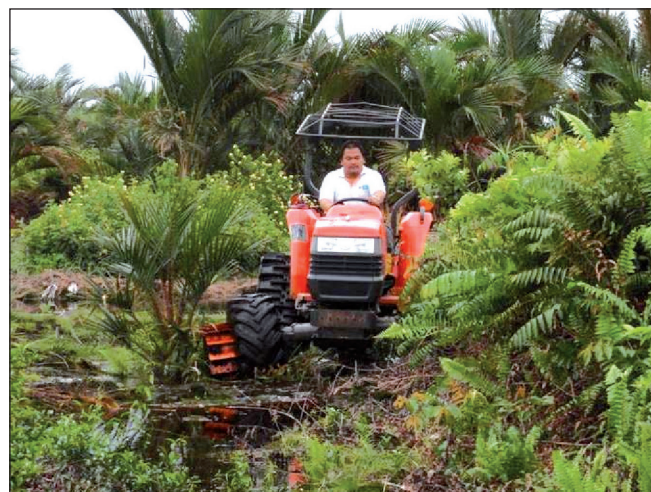
Figure 5. The machine aided with cage wheels successfully maneuvering on peat soil.
