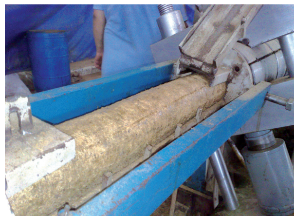
Figure 1. Piston press technology used in the production of palm biomass briquettes.
