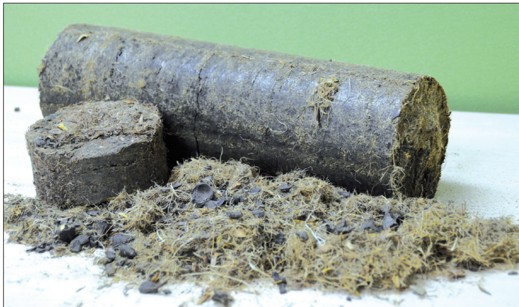
Figure 4. Palm biomass briquettes made from EFB fibre and palm shells.
