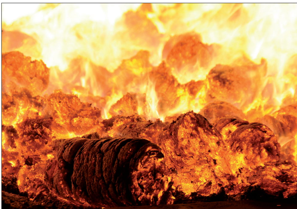
Figure 5. Combustion of palm biomass briquettes in a boiler.
