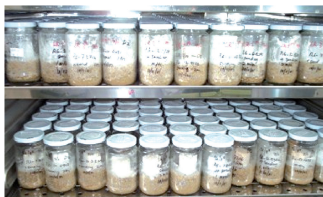
Figure 1. Decaying oil palm trunk test-blocks, each placed on a rubberwood feeder block and inoculated and colonized by different rotting fungi in a standard rotting experiment. Each row of six bottles (from back to front) was inoculated with the same fungus. There were 22 rows of bottles inoculated with 22 different rotting fungi; they were incubated for three months.
