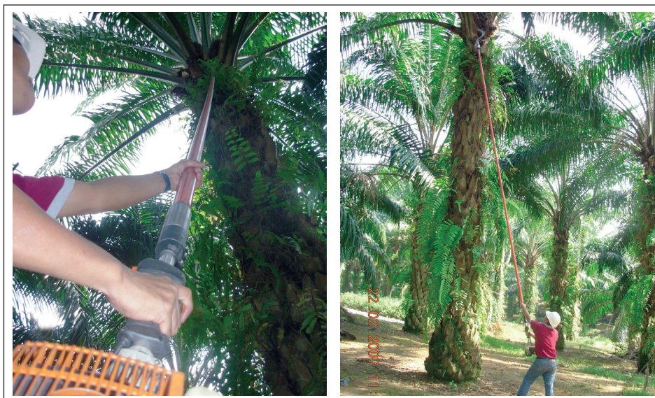
Figure 1. Cantas7 in operation.
