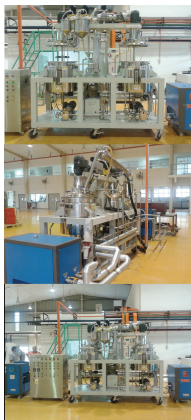
Figure 1. The 150 litres polyol pilot plant.
