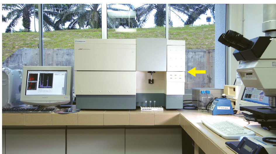
Figure 1. FACS Calibur (Becton Dickinson, USA) Flow Cytometer (yellow arrow). The monitor on the left is displaying fluorescent intensity histogram peaks of nuclei stained with propidium iodide captured by the CellQuest software.
