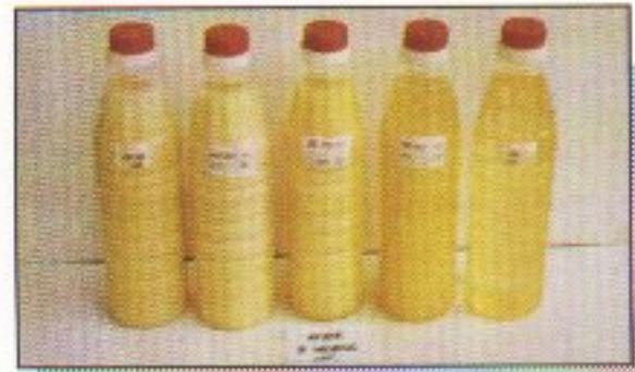
Figure 4(a). Cold stability of blends of single fractionated palm olein with sunflower seed oil after three months at 10°C. The blends are those listed in Table 1, with (L to R) 100%, 70%, 50%, 30% and 0% of palm olein.
