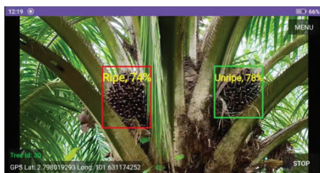
Figure 1. I.M.B.A.S., an AI-based FFB ripeness detection system.
