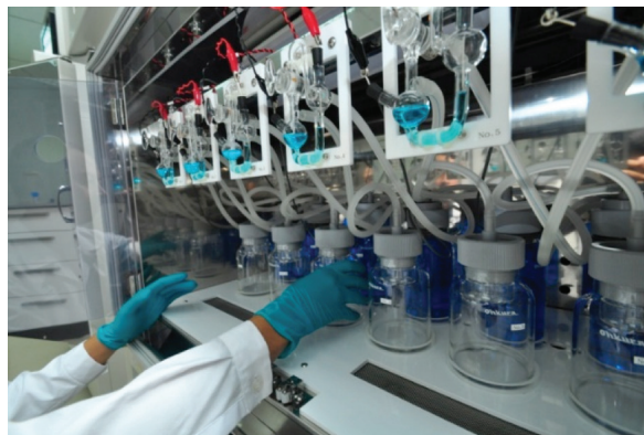
Figure 2. Coulometer used to measure biodegradation.
