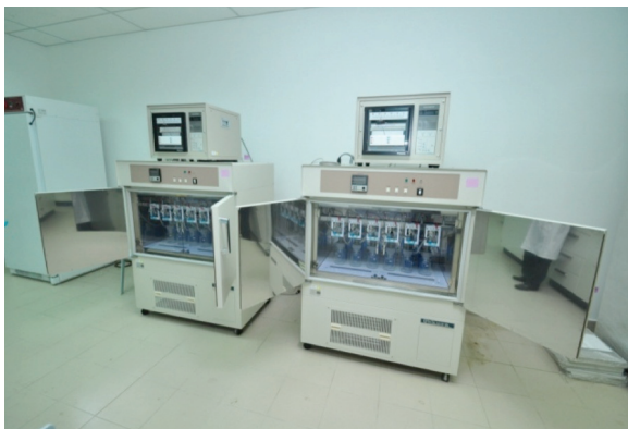
Figure 2. Coulometer used to measure biodegradation.
