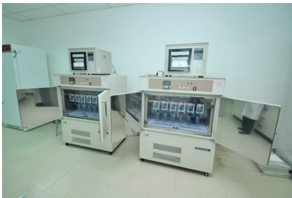
Figure 2. Coulometer used to measure biodegradation.
