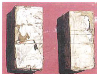
Figure 2. Colonisation of RWB (size 3x3x6cm) with Ganoderma , 2.5 months after incubation at 28°C.
