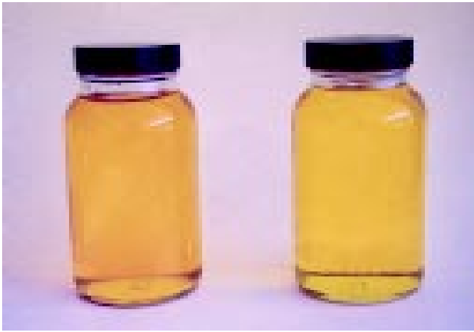
Figure 4. (a) Crude palm kernel oil extracted from shell free palm kernel (right); (b) Crude palm kernel oil extracted from existing commercial palm kernel (left).
