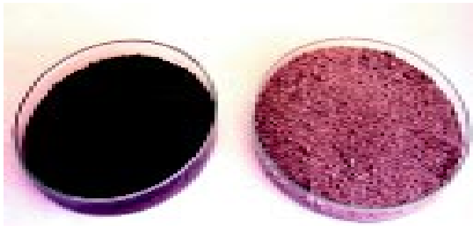
Figure 5. (a) Palm kernel cake produced from shell free palm kernel (right); (b) Palm kernel cake derived from existing commercial palm kernel (left).
