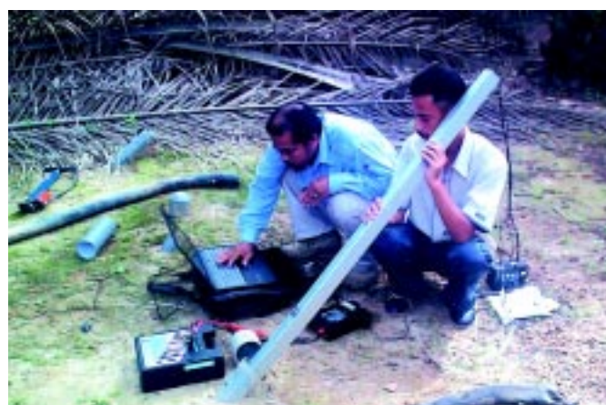
Figure 2. Capturing root images from a PVC observation tube (OT) after removing the motorcycle inner tube (MT).
