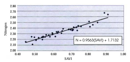
Figure 4. Foliar nitrogen versus SAVI with linear fit line.
