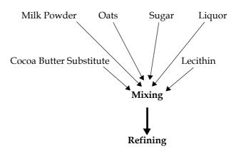
Refining involves the crushing, milling and shearing of cocoa and sugar fragments to produce a product, which has the desired particle size. Only an even particle size distribution gives the required optimum viscosity/yield value and taste.
