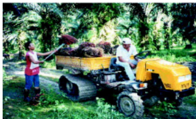
Figure 1. A half-track machine being tested in an area where a wheeled-type vehicle would have poor traction.
