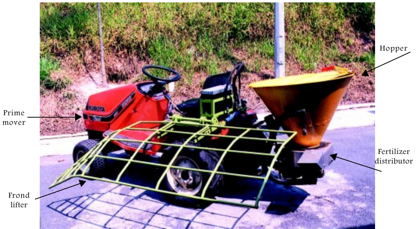
Figure 1. The mechanized fertilizer spreader for young palm.
