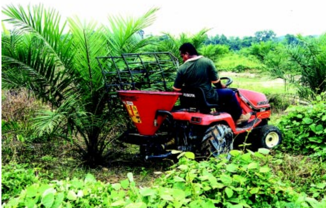
Figure 2. Mechanical fertilizer spreader in action.
