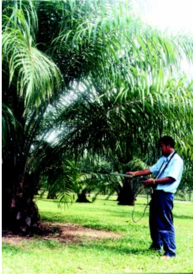
Figure 4. Below canopy reading using the LAI-2000.
