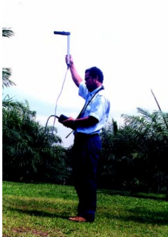
Figure 3. Above canopy reading using the LAI-2000.
