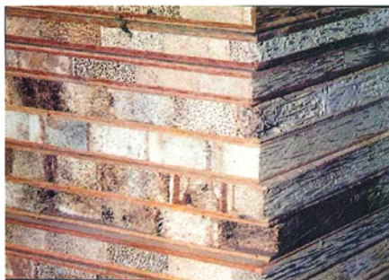
Figure 1. Blockboard from oil palm trunk.
