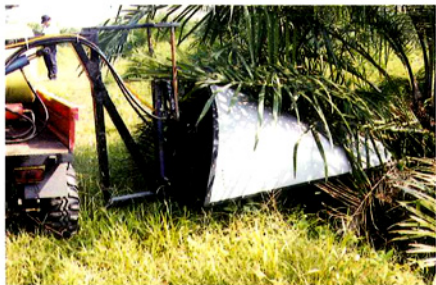
Figure 2. Spray cover eliminates the spray drift affecting the fronds.
