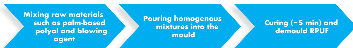
Figure 1. General process of preparing rigid polyurethane foams (RPUF).
