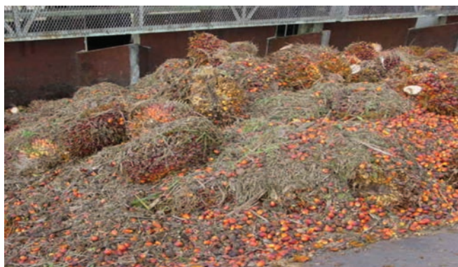
Figure 1. Foreign materials and debris mixed with FFB and loose fruits at hopper.
