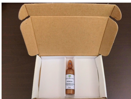
Figure 1. PKO RM are supplied in 5 ml amber-coloured glass ampoules.
