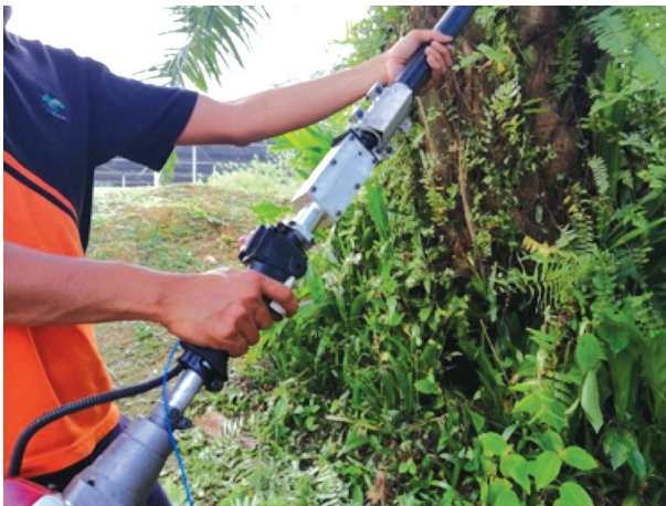
Figure 2. Vibration measurement at throttle point (left) and pole point (right).
