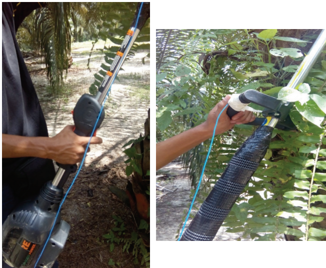
Figure 4. Vibration measurement at throttle point (left) and pole point (right).
