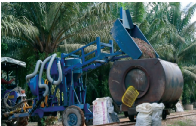
Figure 5. Unloading loose fruits into steriliser cage.
