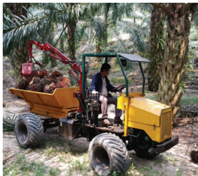
Figure 2. A 4-wheel transporter during field test.
