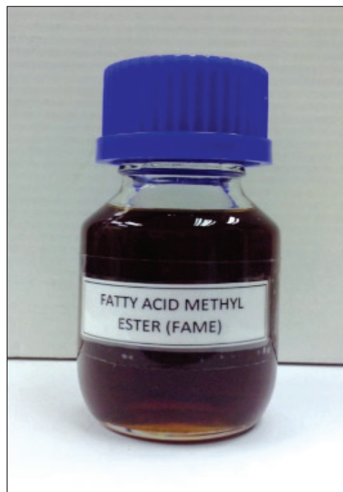
Figure 1. Fatty acid methyl ester (FAME) produced from palm fatty acid distilled (PFAD) via glycerolysis process.
