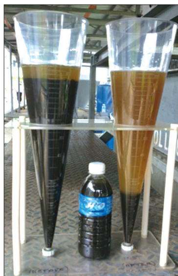
Figure 4. Palm oil mill effluent samples: (a) before and after micro-screening filtration; (b) after membrane ultra-filtration.
