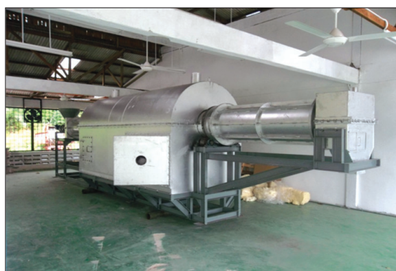
Figure 1. The prototype of the rotary kiln system for continuous carbonisation and the commercial specifications.
