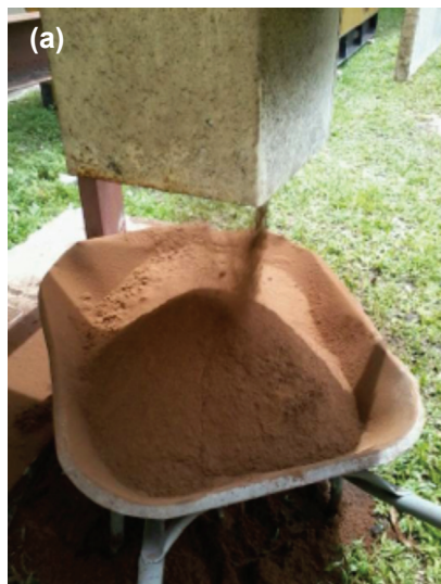
Figure 2. (a) The powdered PKS produced from the Nanomass System, and (b) the size distribution analysis of the powdered PKS.
