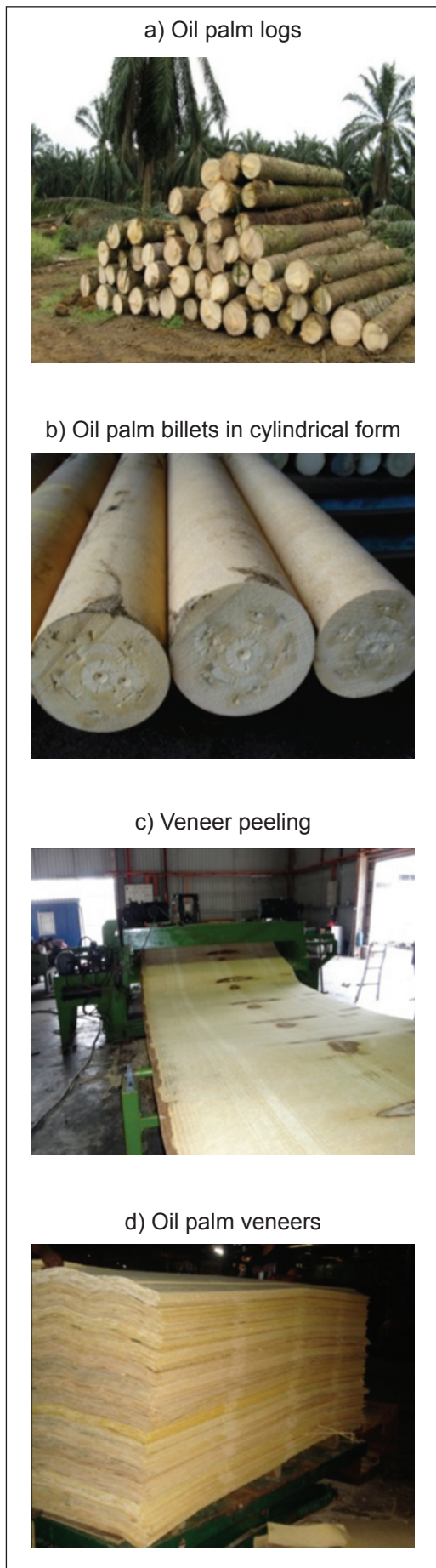
Figure 2. A process flow of the major stages for the veneer peeling operations from oil palm logs.
