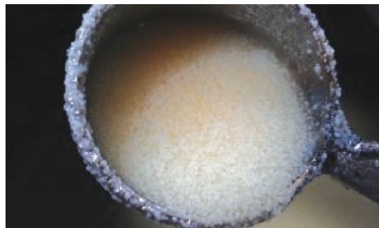
Figure 2. Slurry using MPOB modified recipe. Note the more uniform crystal size with a smaller mean size.
