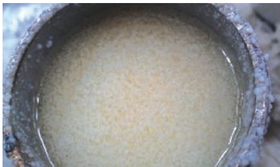
Figure 1. Slurry using refinery recipe. Note the less uniform crystal size with a larger mean crystal size.
