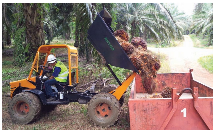
Figure 3. Unloading of bunches into bin.
