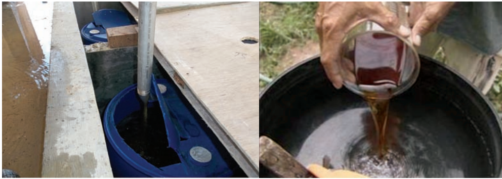
Figure 2. The condensation and collection of palm-based pyroligneous acid.
