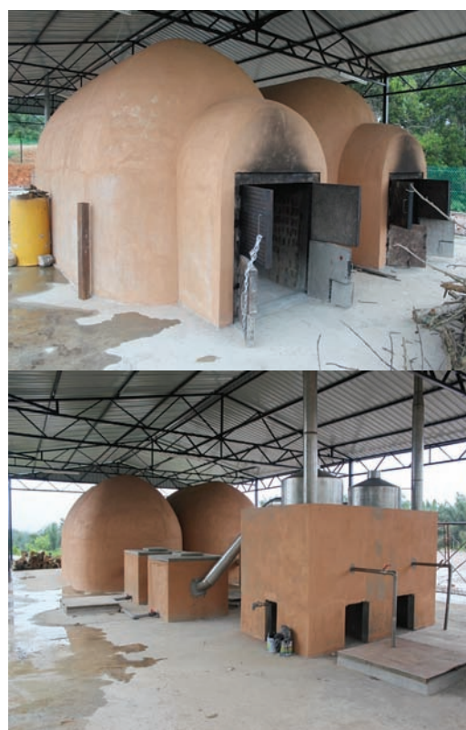
Figure 1. The kiln and the condensation chambers of the system.
