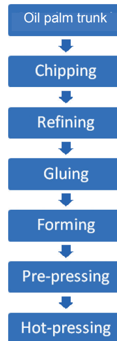
Figure 1. Process flow of MDF manufacture from oil palm trunks.
