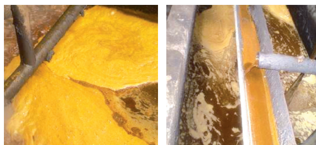
Figure 3. Oil extracted by RORS being recovered at the oil recovery tank in the palm oil mill.
