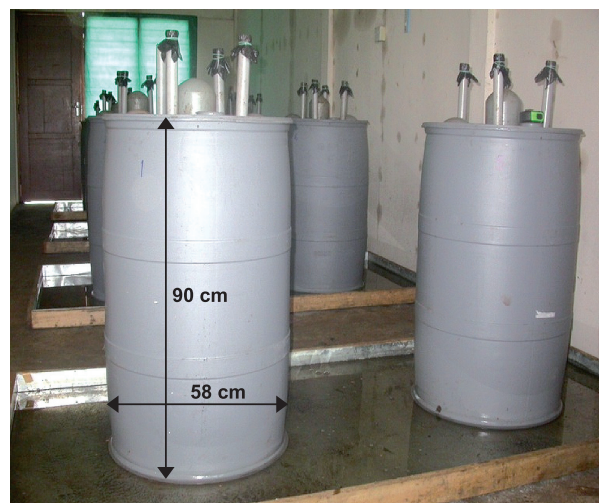
Figure 1. Lysimeters made from high-density polyethylene (HDPE) tanks filled with peat soil to which were introduced the pest termite species, Coptotermes curvignathus , for the water-table study at 15, 30, 50 and 70 cm from the soil surface.
