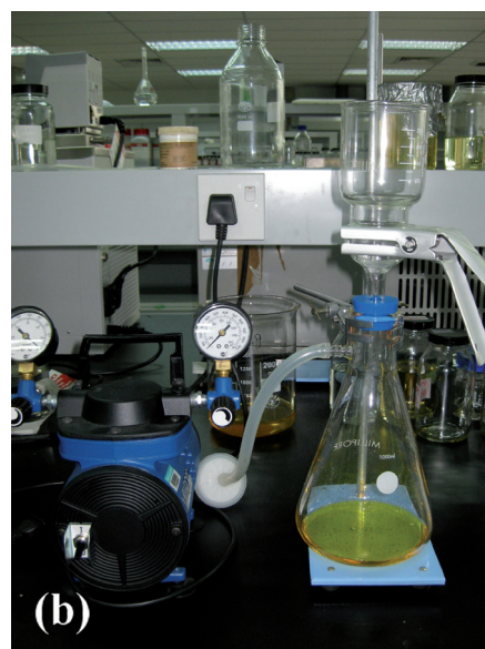
Figure 1. Equipment set-up for the cold soak filterability test. (a) Sample conditioning, (b) filtration system.
