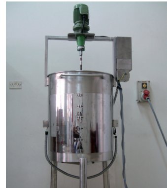
Figure 2. A 200-litre capacity mixer tank for blending of palm-based mould oil.
