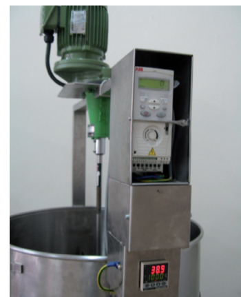
Figure 3. Agitation and heating system of the mixer tank.
