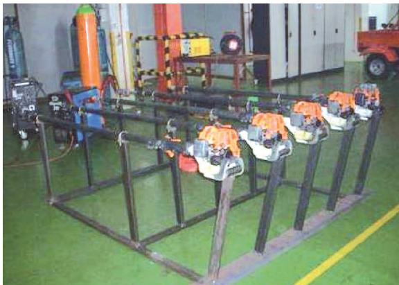
Figure 4. Endurance and fatigue test jig.
