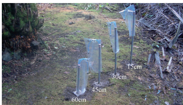
Figure 3. A set of lysimeter tubes installed in the palm circle at four soil depths: 15, 30, 45 and 60 cm.
