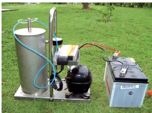
Figure 2. Battery-operated vacuum pump (which provides a vacuum of up to -76 cmHg or -1.01bar).
