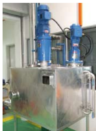
Figure 1. Stainless steel pilot-scale soap reactor.
