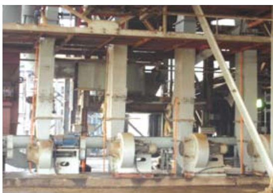
Figure 1. The four-stage winnowing column.
