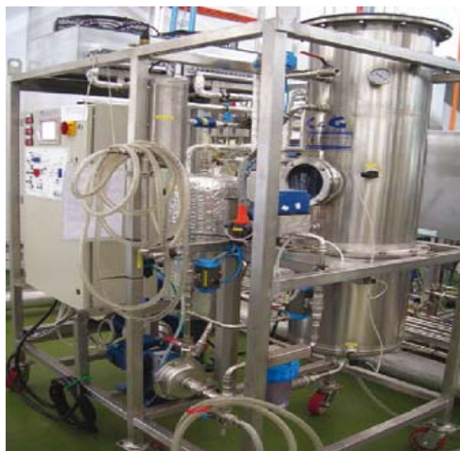
Figure 2. MPOB pilot plant vacuum evaporator.
