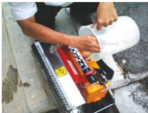
Figure 3. Bafog-1(S) solution was mixed and poured into 7 litres solution tank.
