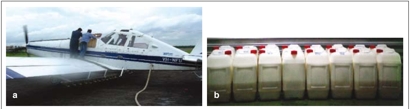
Figure 6. Water being pumped to dilute the Ecobac-1 (EC) poured inside solution tank of the aircraft (a) and (b) Ecobac-1 (EC) in 25 litres containers for field application.
