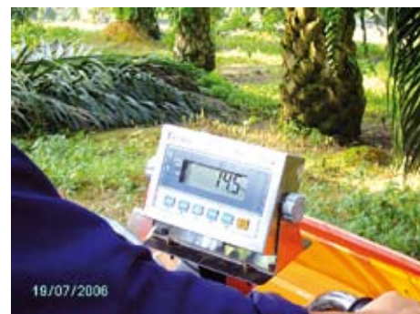
Panel display automatically showing the accrued weight of bunches.
