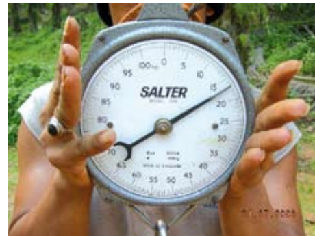
Bunch weight displayed on spring balance.
