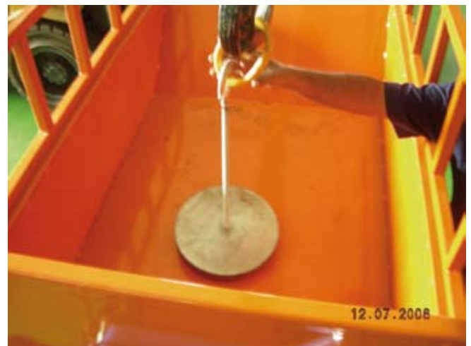
Figure 2. A known weight placed in the bucket for calibration.
