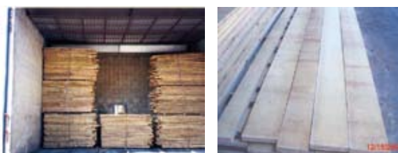
Figure 1. Oil palm lumber drying in the kiln drier.
