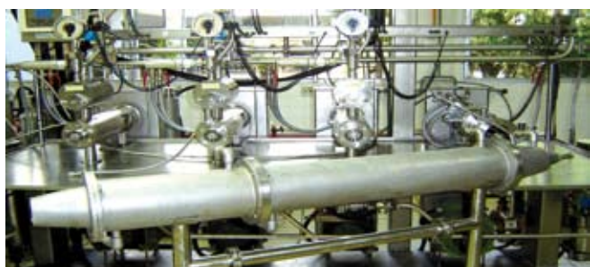
Figure 2. Perfeqtor pilot plant with the resting tube.
