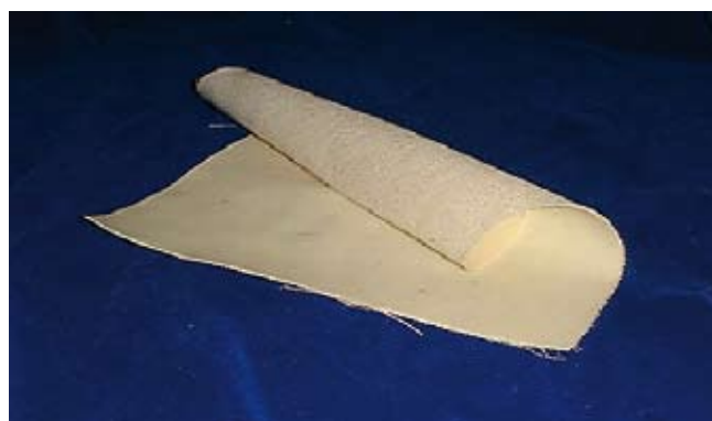
Figure 3. Polyurethane sheet laminated with gauze.
